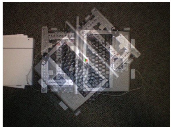
Figure 3: An uncalibrated supposedly 90° turn on the new hybrid OmniWheel drive system in the hall. Note the actual turn is 135° but there is almost no translation. The laptop power button colored red and green is almost over the exact center of rotation.
