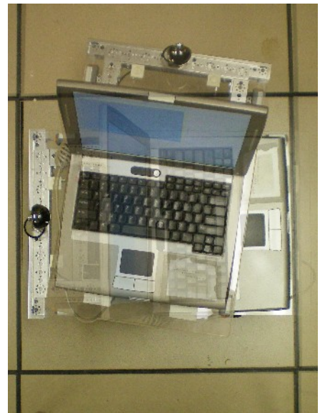
Figure 1: A supposedly 90^\circ turn in the Robotics Lab using the old drive system. Note the actual turn of 100^\circ and the considerable drift toward the top of the image.
